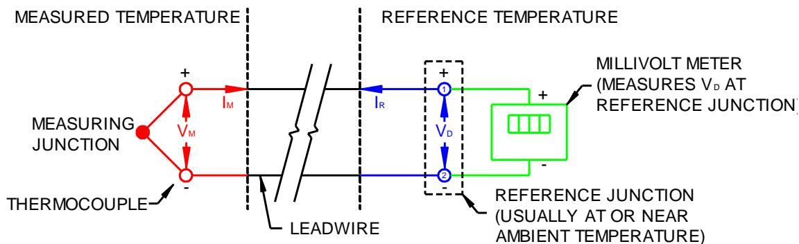
**HOW TO DETERMINE THE MEASURING JUNCTION TEMPERATURE**
