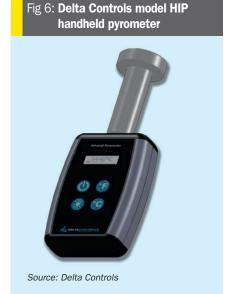
A portable pyrometer designed for use in a Claus thermal reactor (Fig. 6) will have the appropriate narrow field of view, will detect the same wavelengths of light as the permanent pyrometer, and will ignore the attenuation of the window or any partial bore occlusion.
