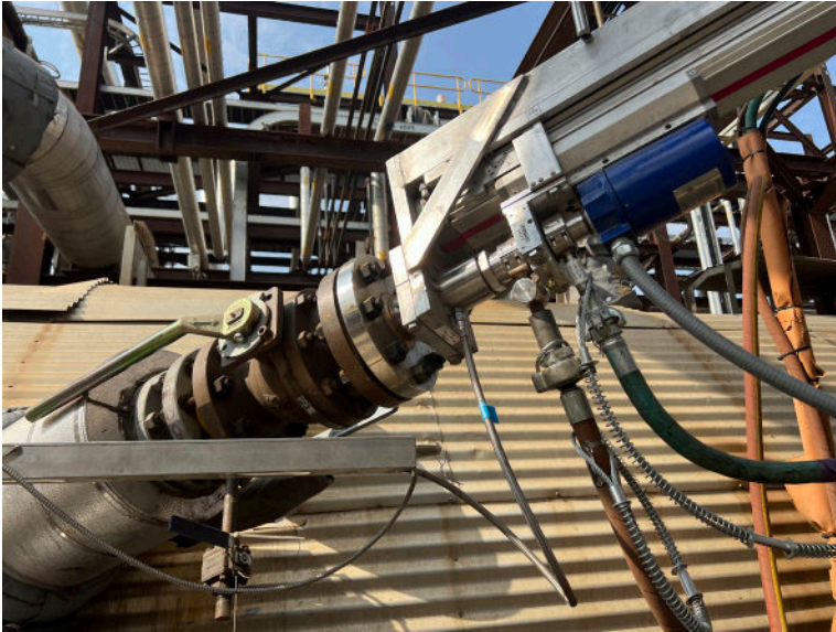
Figure 2. The extractor and probe assembly bolted to the vessel's isolation valve and required utilities established.
