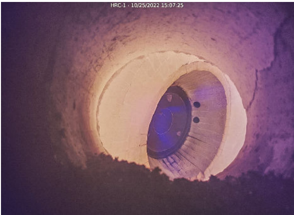
Figure 3. First image produced showing material deposition along the test nozzle bore.
