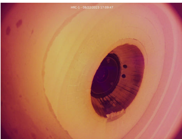
Figure 4. The process camera provides online images of the burner, refractory lining or tubesheet protection system.
