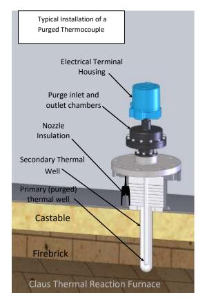
the specially designed nozzle insulating materials. Weld neck flanges make ideal nozzles since they have no weld beads in the ID that often restrict insertion of solid insulating rings.
