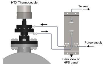
Thermocouple failure is most often the result of process gases contacting thermoelement wires. In general, the rate at which the thermocouple fails is directly related to the amount of exposure the thermocouple has to the process gases. A broken thermowell usually causes thermocouple failure within days or months. A purge supply loss may go unnoticed for months while the thermocouple output slowly degrades. Failure can be caused by a variety of reasons:
