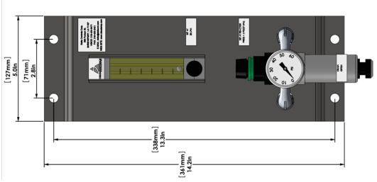
PIPING OR TUBING MAY ARRIVE AT THE HFI STATION HORIZONTALLY (FROM THE RIGHT AND/OR LEFT), VERTICALLY (FROM UP AND/OR DOWN) OR ANY COMBINATION OF THESE DIRECTIONS. CONNECTION FITTINGS MAY BE ROTATED  $\pm 200^\circ$ . FIELD CONNECTIONS:
