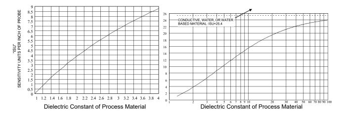
STEP #3 INSERT "BSU" AND "ISU" (DETERMINED ABOVE) INTO THE FORMULAS SHOWN IN APPLICATION NOTE # PROB-198; "FORMULAS FOR MODELING AND PERFORMANCE TESTING". VERIFY THAT THE SELECTED PROBE AND ELECTRONICS MODULE WILL MEET THE REQUIREMENTS OF THE APPLICATION AND PROVIDE THE EXPECTED RESULTS.
