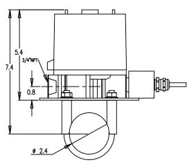
Hot Lens Assembly / Steam Fixture / Process Connection Orientation
