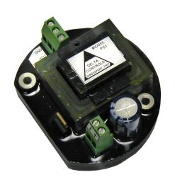
FOR STACK MOUNTING; SIGNAL LOOP POWER SUPPLY. THE MODEL PS CAN DRIVE 3 SWITCHING RELAY POINTS OR 6 SIGNAL LOOPS.
