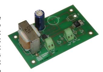
FOR MOUNTING IN A NEMA BOX IN PLACE OF A BACKPLATE. IT CAN DRIVE 3 LOOPS OR 1 LOOP AND AN ALARM RELAY MODULE.
