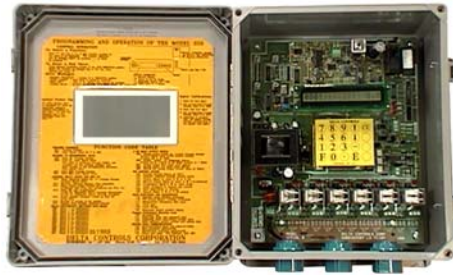
MODEL 858 SMART TRANSMITTER, 6 RELAYS
