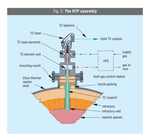
internal passages of the thermocouple. A slight elevated backpressure of the flush gas is maintained by the use of a flow meter equipped with a flow control valve located at the purge outlet. The purge function is most easily accomplished with the use of a convenient "flush gas" control station equipped with the pressure regulator, filter, drip well, flow meter and valve.
