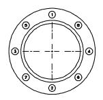
This shows the recommended tightening sequence of the flange bolts (lubricate threads)
