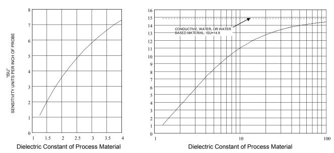
STEP #3 Insert "BSU" and "ISU" (determined above) into the formulas shown in Application Note # PROB-198; "FORMULAS FOR MODELING AND PERFORMANCE TESTING". Verify that the selected probe and electronics module will meet the needs of the application and provide the expected results.
