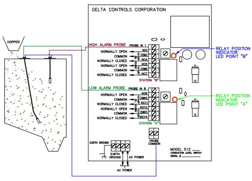
SHOWN: STATION "A" WIRED AS LOW LEVEL POINT ALARM STATION "B" WIRED AS HIGH LEVEL ALARM
